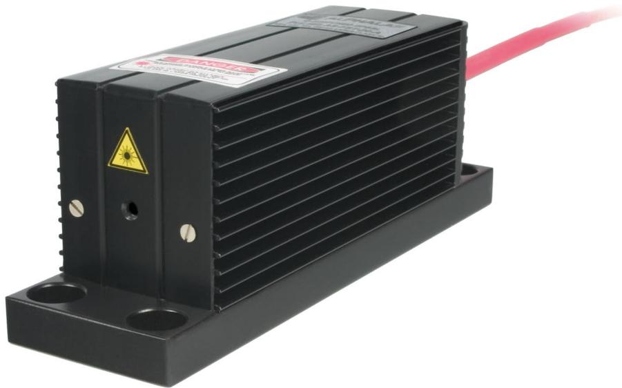
A wide range of passively Q-switched lasers with pulse durations below 1 ns and extremely high peak powers at 1064 nm with excellent TEM<sub>00</sub> beam profile are offered by ALPHALAS. The PULSELAS®-P lasers feature proprietary microchip design. The monolithic laser cavity is permanently aligned and therefore extremely stable.
